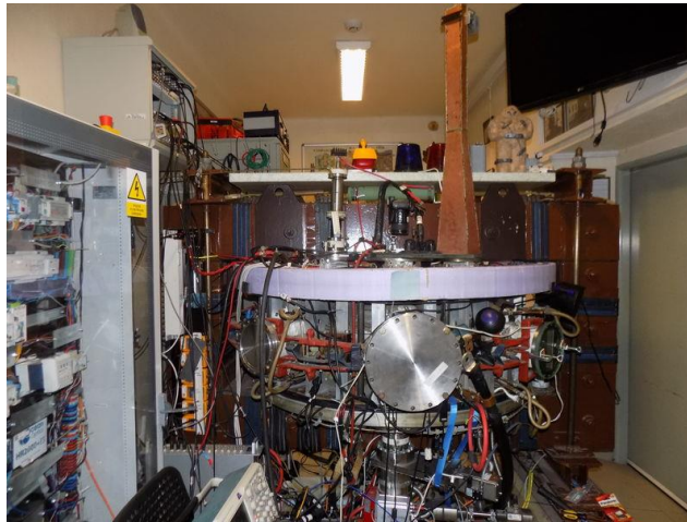
FIG. 1. Tokamak GOLEM equipped with cryostat and MW launcher
