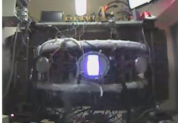
FIG.2. Plasma pulse in the GOLEM tokamak with HTS poloidal field coils.
