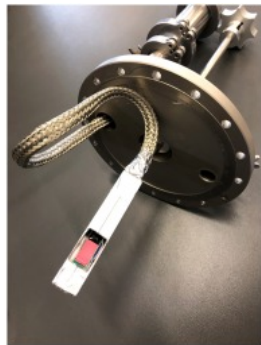
(b) PH32 detector attached to a radial manipulator, used during RE related GOLEM campaigns.
