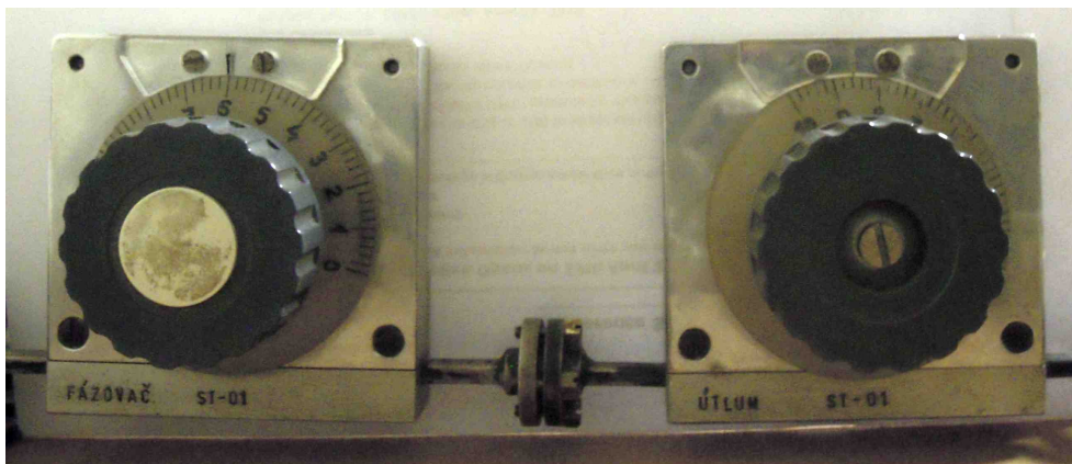
Figure 3.15: Attenuator and phase shifter (reference wave path)
