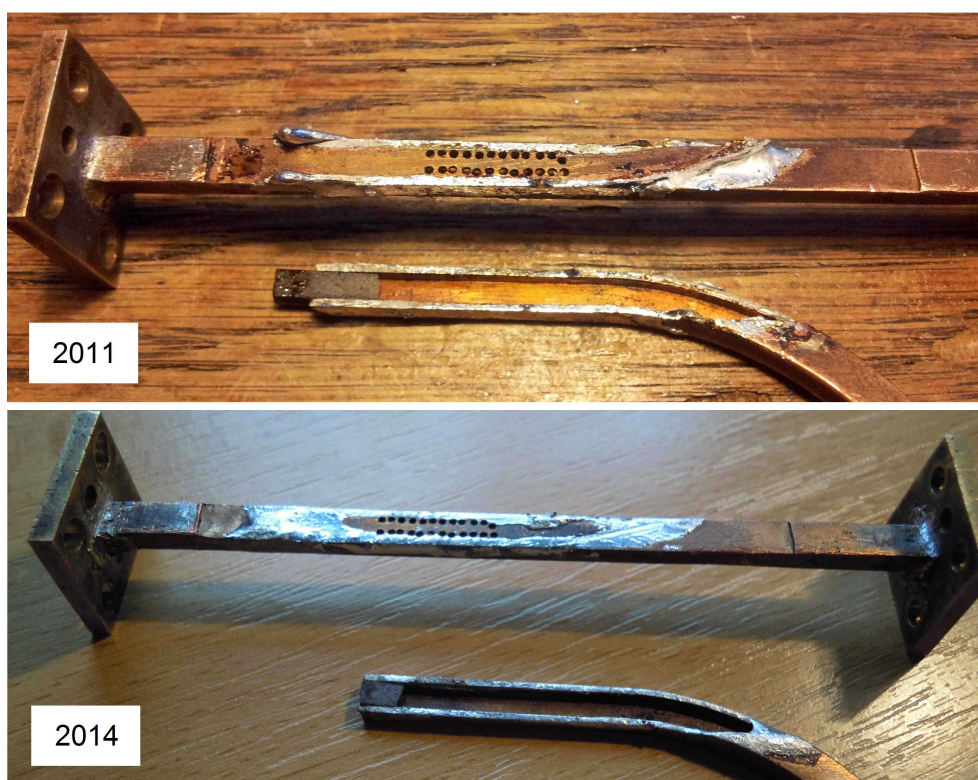
Figure 3.13: Directional coupler - desoldered
