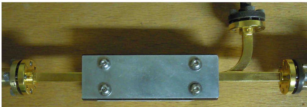
Figure 3.14: New directional coupler with its protective support
