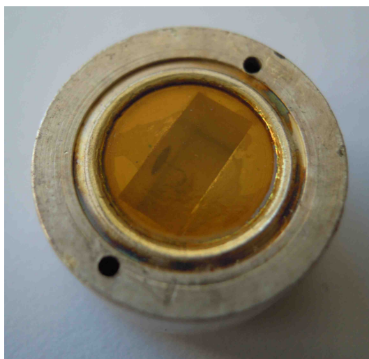
Figure 2.4: D-404 detection diode (waveguide dimensions are about 7.1x3.55 mm – Ka band)
