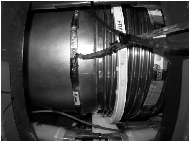
FIG. 2. Diamagnetic coil assembly mounted in STOR-M (center, white form mounted on bellows). Also in the picture at the bottom is one of the structural mounts physically isolating the coil from the vacuum chamber.
