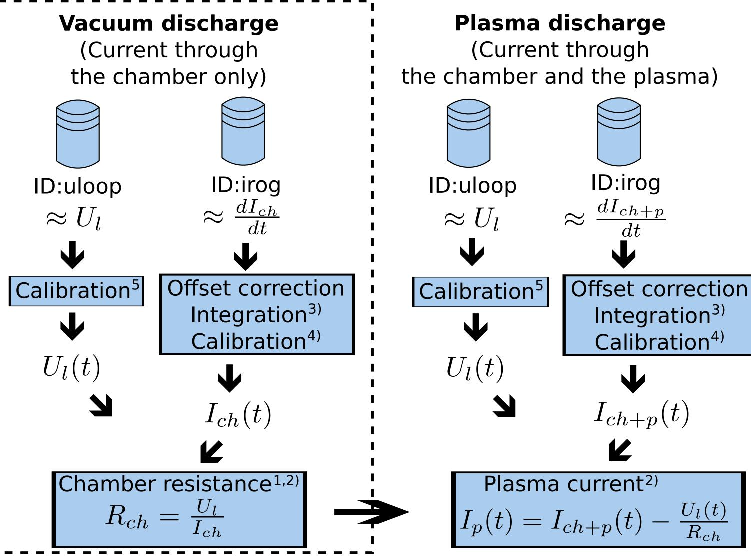
1) With some statistical effort. 2) Do it in the stationary phase, i.e. current constant, to avoid inductive phenomena. 3) 1 us step. 4) Rogowski Coil calibration constant = 5.3 . 10<sup>6</sup> A/Vs 5) Uloop calibration constant = 5.5
