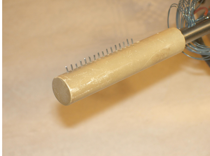
Figure 4: The rake probe on GOLEM. It is made of 16 Langmuir probe pins. Only 12 probes are measuring due to the number of available acquisition channels. These probes are measuring the floating potential at different radial location from the centre of the plasma to the plasma edge. Two consecutive probes are separated by 2.5 mm.
