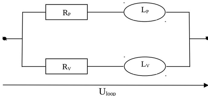
where  $R_p$  and  $R_v$  are the plasma and the vessel resistivities and  $L_p$  and  $L_v$  are the plasma and the vessel inductances.  $R_v$  and  $L_v$  are characteristic of the vessel and thus independent of time. Note that the loop voltage  $U_{loop}$  is measured directly.
