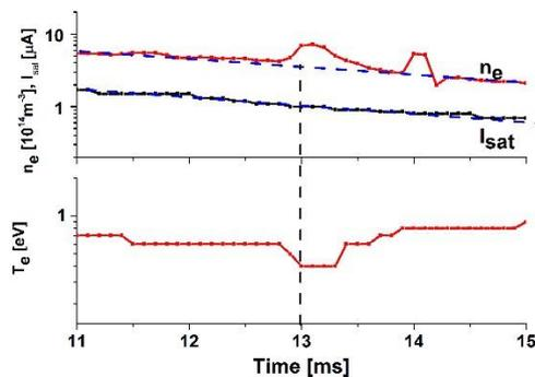
**Fig. 4.** Evolution of selected plasma parameters in the time interval when MW power is switched off. The  $I_{sat}$  and  $n_e$  decay exponentially with the characteristic time constant
