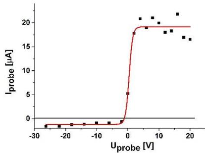
**Fig. 2.** IV characteristics constructed at  $t = 12$  ms, when the toroidal magnetic field is  $B_0 = 0.188$  T.
