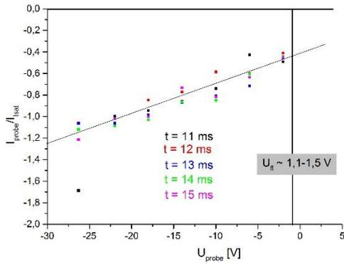
**Fig. 6.** Ion branch of IV characteristics at  $t = 12, 13, 14,$  and  $15$  ms, normalized to the  $I_{sat}$  resulting from the analytic fits.
