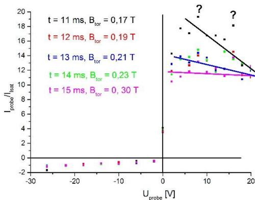
**Fig. 7.** IV characteristics at  $t = 12, 13, 14,$  and  $15$  ms, normalized to the  $I_{sat}$  resulting from the analytic fits.
