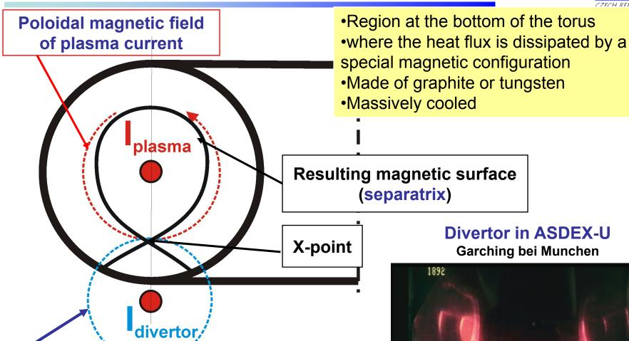
Poloidal magnetic field of an external toroidal loop with the electric current in the same direction as the plasma current
