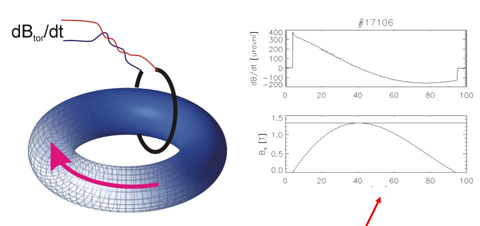
Signal of the loop has to be integrated
