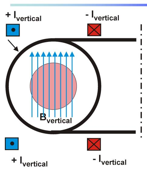
Vertical magnetic field is generated by four loops with defined direction of current
