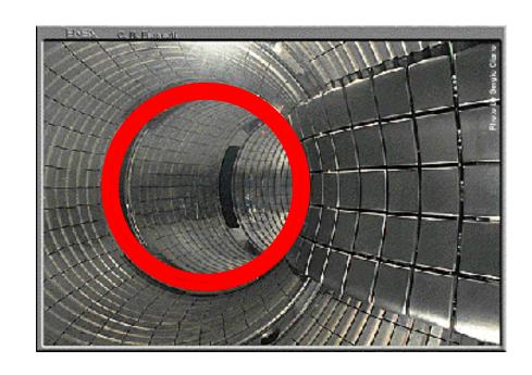
Poloidal limiters were exploited in the first generation of tokamaks
