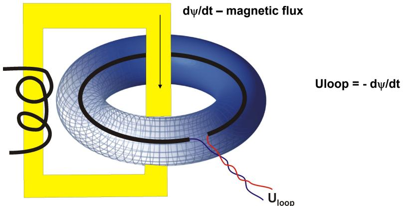
The loop voltage is measured by a loop located in the proximity of the plasma column
