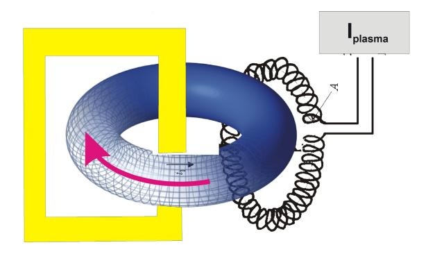
Plasma current is measured by means of the Rogowski coil (the solenoid of a toroidal shape surrounding the plasma column)
