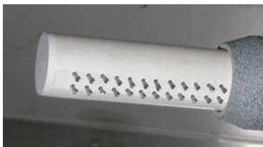
Fig. 3. Photograph of the double rake probe. Two rows of Langmuir tips are spaced poloidally by 2.5 mm. The radial distance between the tips is also 2.5 mm. The individual tips measure either the floating potential or the ion saturation current. The mode of operation can be changed between shots. Signals are recorded with the sampling frequency 1 MHz
