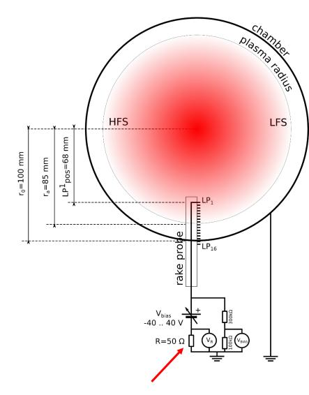
Radial array of 16 Langmuir tips is immersed in the plasma from the bottom of the tokamak vessel, movable on the shot to shot basis.
