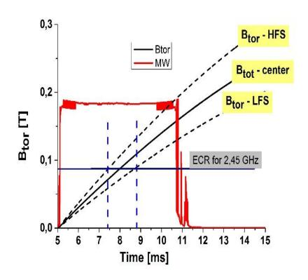
Electron Cyclotron Resonance appears in the vessel for the time interval  $^{\sim}1,5$  ms, when the toroidal magnetic field is Bt = 0. 087 T
