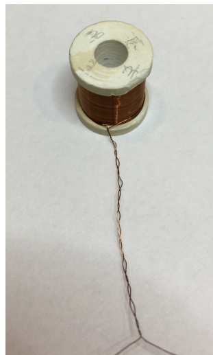
Figure 3.29: Constructed coil with twisted end.
