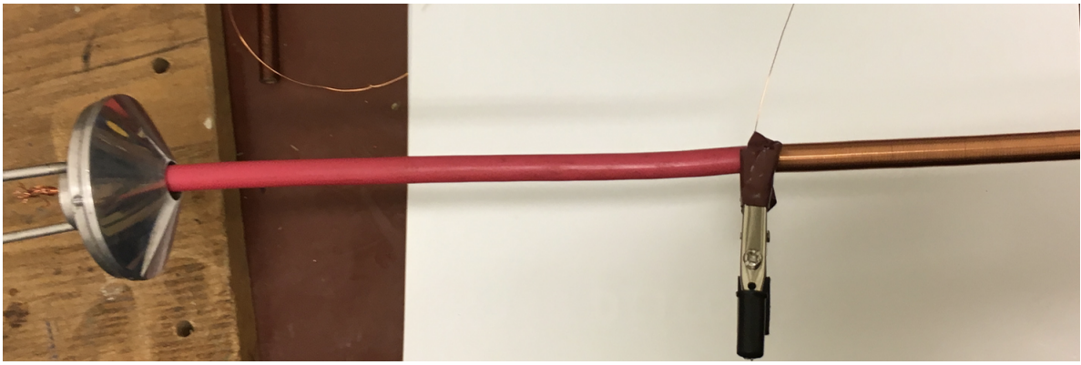
Figure 3.36: Half wound Rogowski coil using a d = 0.25 mm copper wire.
