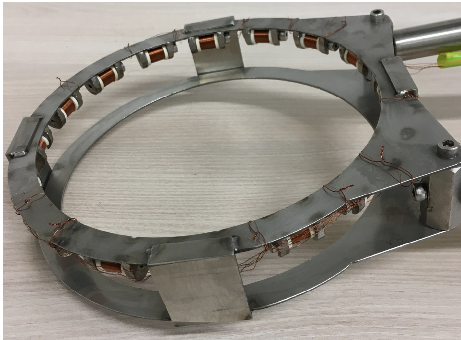
Figure 3.31: Set of 16 Mirnov coils installed in the assembly ring.
