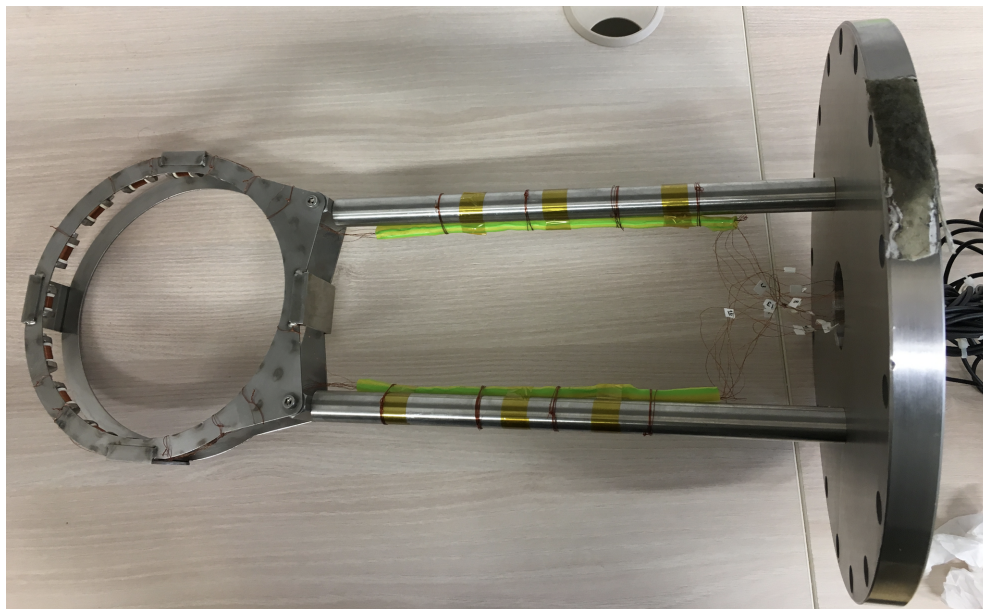
Figure 3.33: Complete assembly with 16 Mirnov coils installed.
