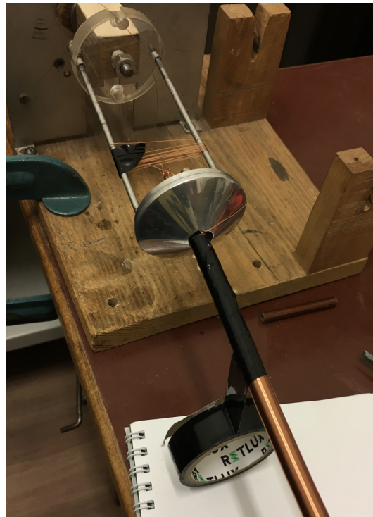
Figure 3.37: Rogowski coil with electric tape wrapping.
