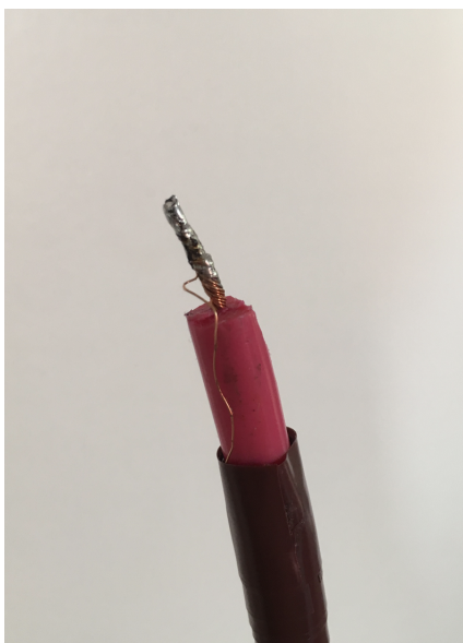
Figure 3.38: Welded ends of the Rogowski coil.
