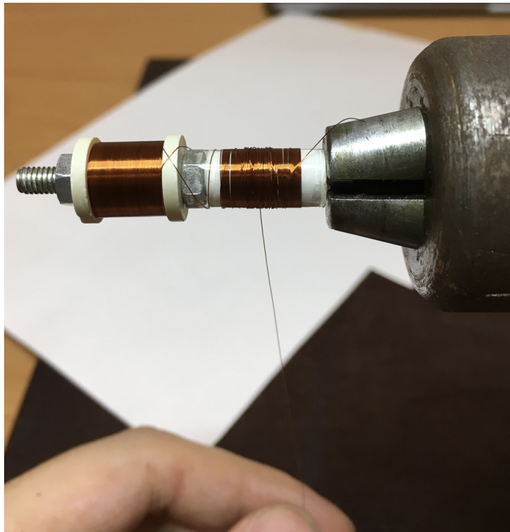
Figure 3.28: Coil and drill system for winding process.
