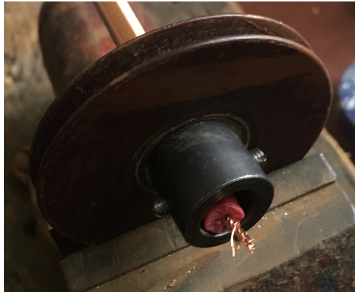
Figure 3.35: Free-rotation bearing fixed at the second end of the thicker cable.
