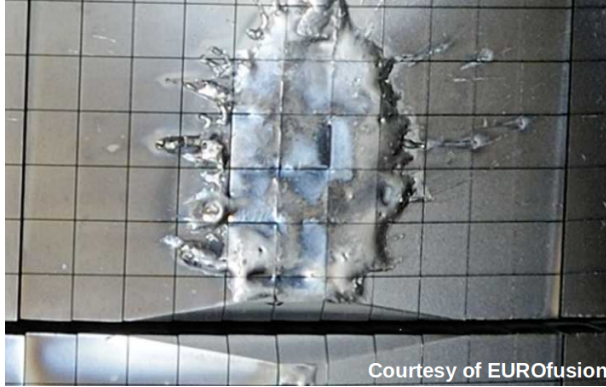
Figure 2.2: Re-deposited molten beryllium at JET ITER-like first wall due to the RE impacts. The picture is copied from Ref. [83].
