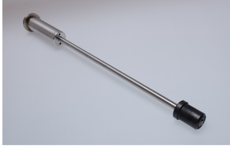
Figure 5.3: The three-channel Cherenkov detector. In the figure the whole set-up of the Cherenkov detector is shown. The detector consists of the measuring head, the detector tube, the detector body and the flange.
