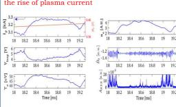
Temporal profile of toroidal electric field  $(E_{\phi})$  normalized with Dreicer field  $(n_e T_e^{-1})$  and  $\dot{B}_{\theta}$  oscillations amplitude for the HXR and non-HXR cases (#27753).
