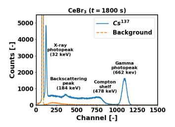
important features of Cs<sup>137</sup> gamma spectrum could be clearly distinguished
