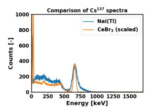
• measured energy resolution  $\approx 6\% @662 \text{ keV}$  (typical value:  $\approx 4\text{-}5\% @662 \text{ keV})$
