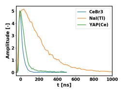
comparison of pulse shape of different detectors: CeBr<sub>3</sub>, NaI(TI), YAP(Ce)
