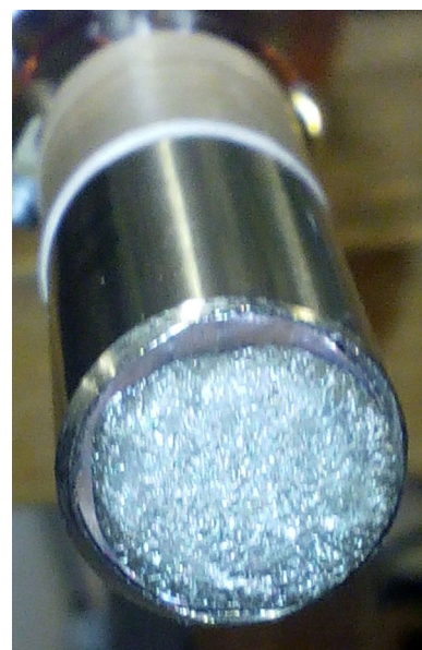
Fig. 2. Tin sample in its holder after exposure to ISTTOK plasmas.
