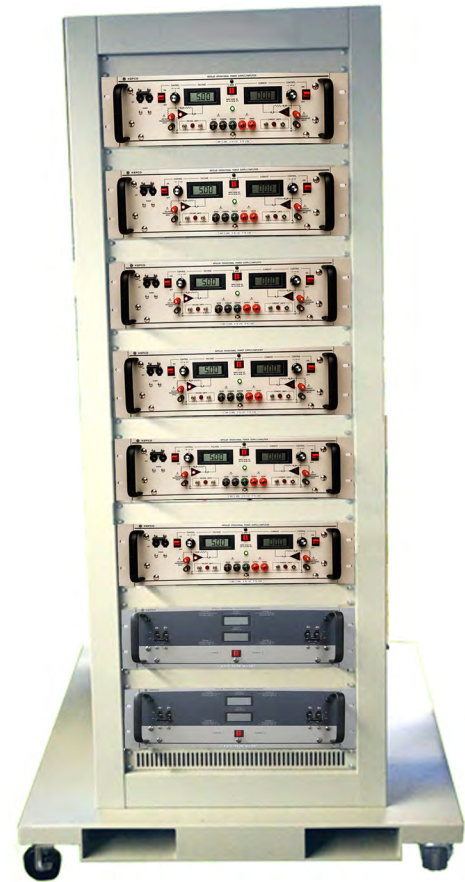
10-Channel Low Power BOP comprised of six 400W channels and four 200W channels
