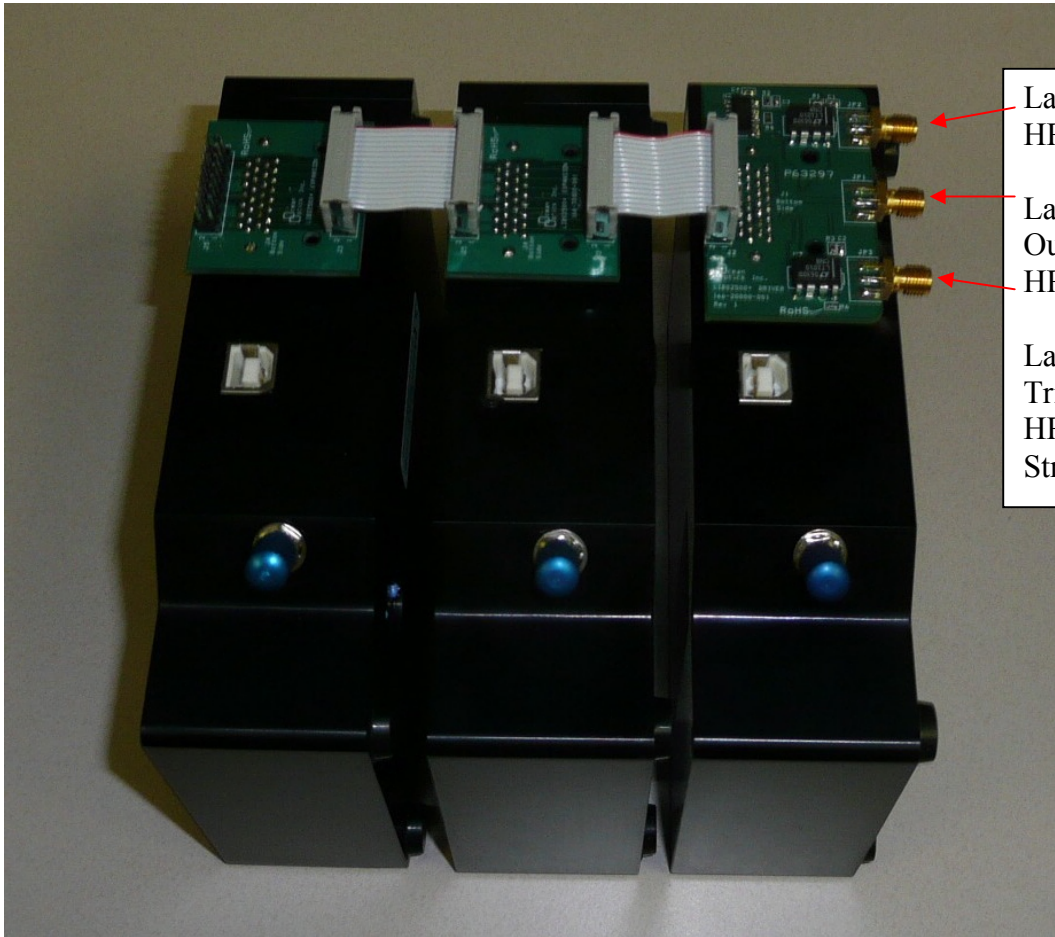
3-channel HR2000+ LIBS setup
