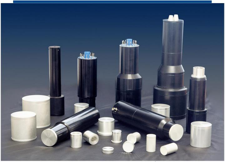
The NuDET NAI series offers a variety of NaI(TI) scintillation detectors with standard shapes and dimensions. The integraly mounted scintillation assemblies are hermetically sealed units containing NaI(TI crystal optically coupled to a photomultiplier The assemblies tube. are designed for crystals up to 3 inches in a diameter. These probes excel with consistent, superior energy resolution and efficiency.
