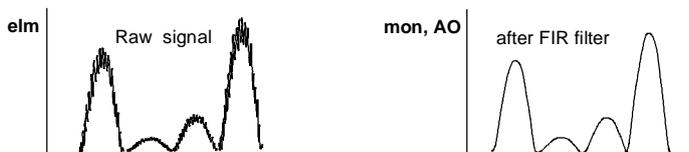
The FIR filter largely eliminates noise and interference so that also very small peaks can be detected against the background. Statistical intensity fluctuations frequently account for the major portion of the noise are particularly well suppressed by the FIR filter. For this reason you should always use *SCAN-F*, except in the few special cases where raw data are actually required.
