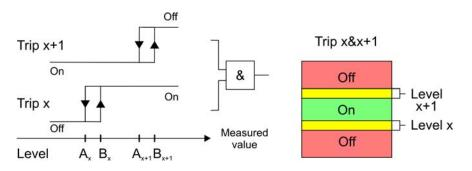
The outputs for "hysteresis" are set when a measurement cycle is finished.
