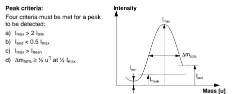
\*)  $\frac{1}{4}$  u with Channels.Parameters.Mass.MassMode = PEAK Time:  $t_{Adjust} \approx 0.5...1.25$  "Dwell"
