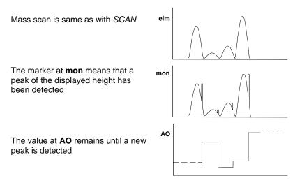
Peak Processing runs with all "Speed" (Channels.Parameters.Mass.DwellSpeed) settings. The peak search extends across the range defined with "FirstMass" and "Width". The peak criteria of General.Cycle.MeasureMode = ADJ\_COARSE apply, see  $\rightarrow B$  66 and following.
