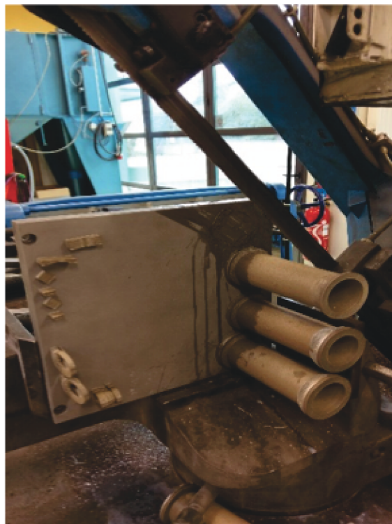
Figure 1. Raw tubes on their support just after printing at BV proto.
