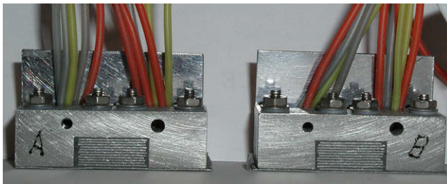
Fig. 2. Photo of the two sides components of the dismantled 'sandwich probe' for measuring the plasma deposition into a gap between tiles. The gap between opposite sides was adjusted to 1.1 mm.
