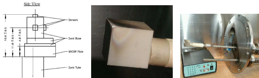
Fig. 1. Left panel: schematic layout of the probe head and distribution of sensors with dimensions. Middle panel: photo of the probe head from outside. Right panel: probe head fixed on the manipulator together with the control electronics box.
