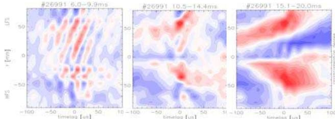
**Fig.3.** Cross-correlation between horizontal chord at 40 mm against all bottom chords prior to biasing (left figure), during biasing with biasing voltage +150V (middle figure) and after biasing (right figure).
