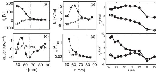
**Fig.2.** Radial profiles of floating potential (a), radial electric field (b), the  $E_r$  shear, (c) ion saturation current (d), toroidal,  $V_\phi$ , (e) and poloidal velocity,  $V_\theta$  (f), averaged over 4 ms before (open symbols) and during (filled symbols) biasing. The vertical line marks the position of the LCFS.
