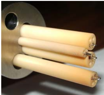
FIGURE 2. Photo of the probe system of ISTTOK, consisting of three emissive probes and one cold cylindrical probe to measure the radial and poloidal electric field and the ion saturation current simultaneously.
