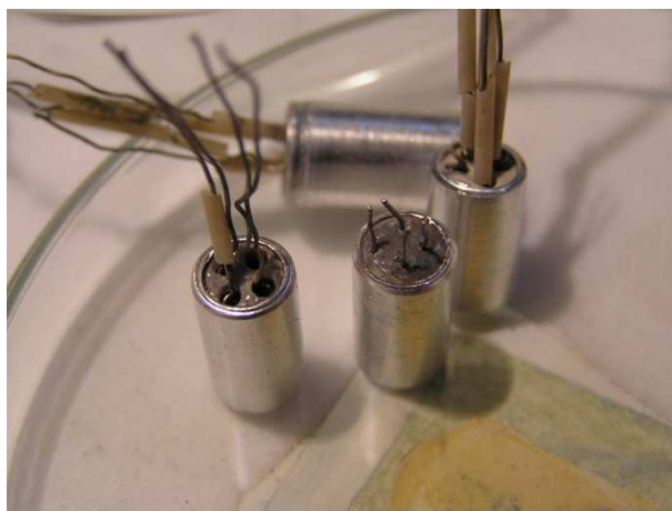
Fig. 4. Sensors taken out from the irradiation head after the full 22 days long irradiation campaign.
