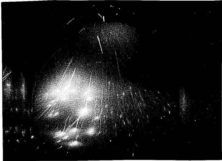
Fig. 11: Photograph showing a sudden path of macroparticles ejected by arcing at a time between 6 and 8 ms after current rise of the tokamak discharge; discharge 14461
