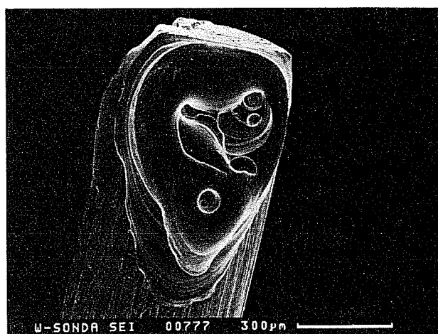
FIG. 7. Traces of local heating at a Langmuir probe.
