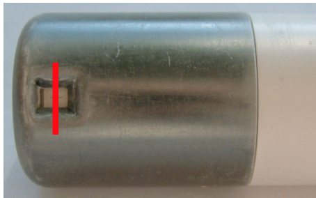
Fig. 4. Photograph of the probe head and the tunnel with slit plate. The vertical red line indicates the shorter of the two rectangular dimensions – this is the section across which the tunnel is simulated.
