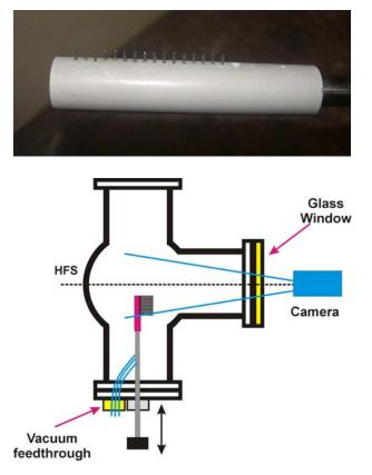
Figure 2: Top panel - probe head containing radial array of 16 Langmuir probes. Bottom panel - schematic layout of experiments with the rake probe on GOLEM tokamak.
