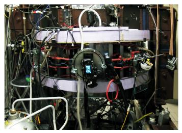
Figure 1: GOLEM tokamak with the visible cryostat housing the pair of high temperature superconducting poloidal field coils.
