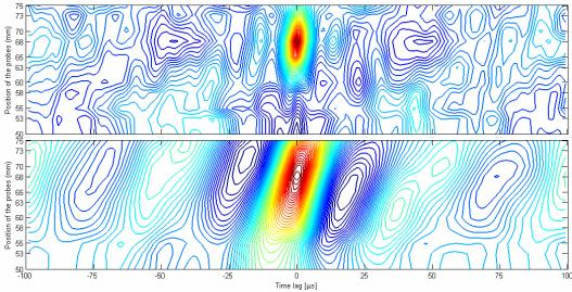
Figure 4: Top panel - cross-correlation functions of  $U_{fl}$  fluctuations in hydrogen plasmas, discharge #9022. Bottom panel - cross-correlation functions of  $U_{fl}$  fluctuations in hydrogen plasmas, discharge #9038.
