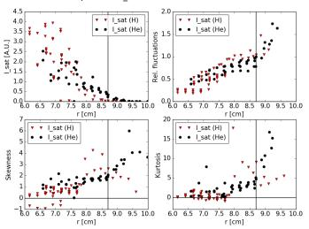
Figure 5: Radial profile of I<sub>sat</sub> fluctuations PDF in hydrogen and helium plasma.
