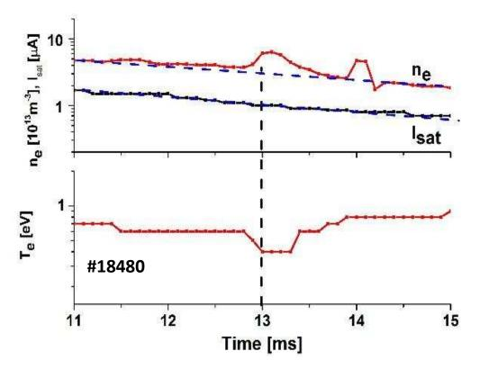
Evolution of the electron density and temperature during MW plasma decay in toroidal magnetic field
