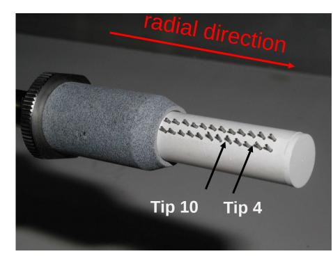
Radial/poloidal distance between adjacent tips is 2,5 mm
