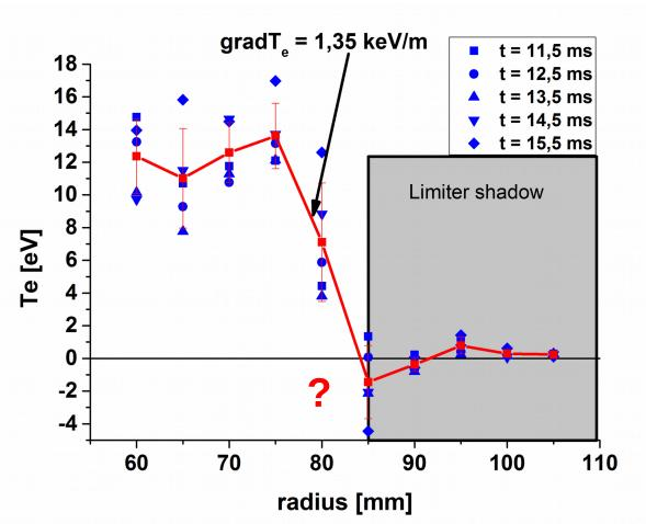
A steep gradient of the electron temperature is formed spontaneously in the proximity of the limiter radius at  $t \sim 10,5 - 11,5$  ms
