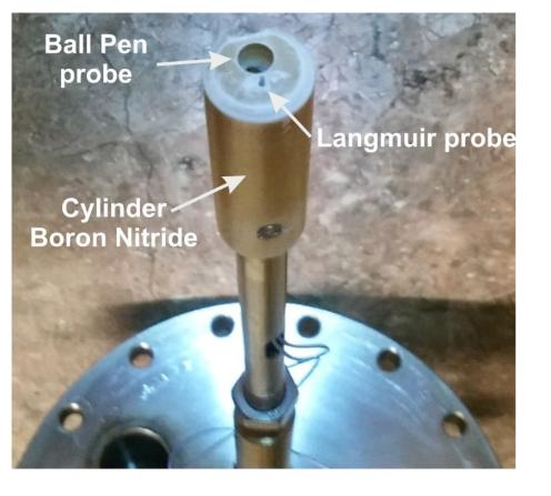
Collector is retracted by 2,3 mm inside the dielectric tube
