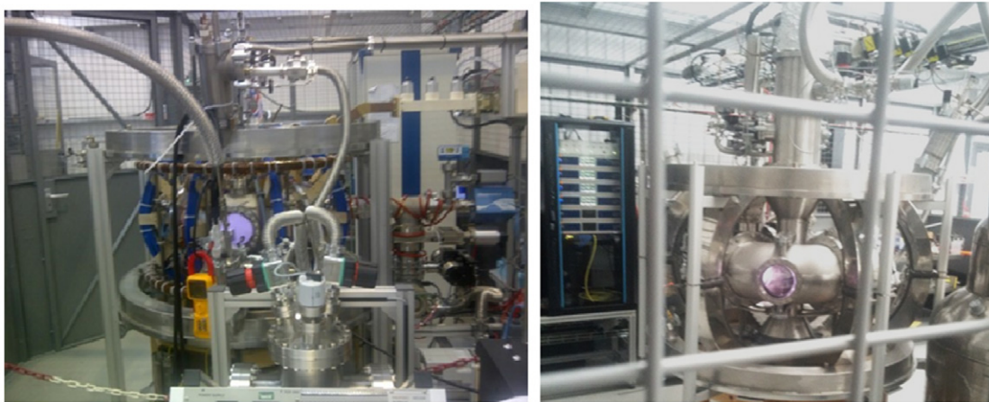
Figure 9. ST25 tokamak with HTS PF coils, left. First plasma in full-HTS tokamak, right.
