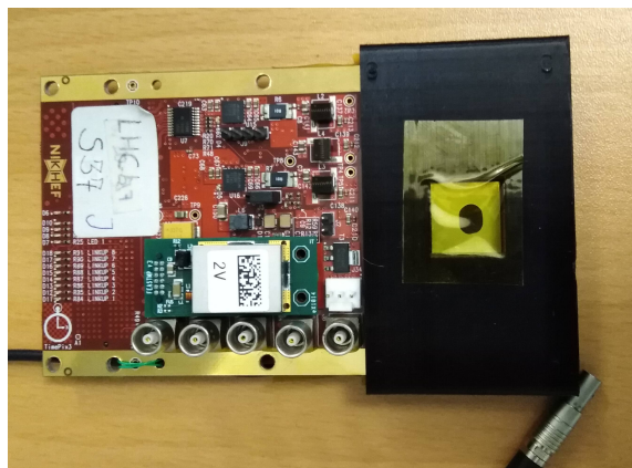
Figure 1. The Timepix3 chipboard. The black plastic is used to shield the Si sensor, which is bump-bonded to the readout ASIC below the sensor, from stray light. Yellow kapton tape keeps the sensor clean from dust. The hole in the Al layer (used for biasing the sensor) atop the sensor was cut out for experiments with a laser at Nikhef.
