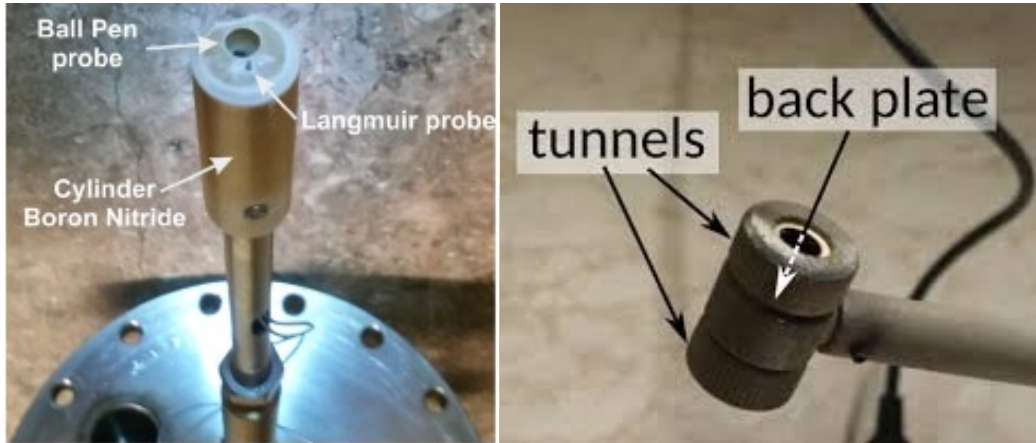
Fig 19: Photos of probes on GOLEM tokamak. On the left – Ball-Pen and Langmuir probe, on the right – double tunnel probe
