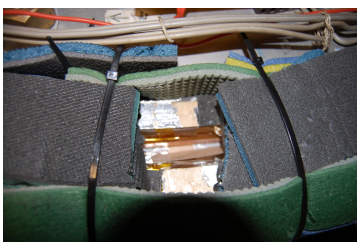
2 x 6 turns of the 2nd generation HTS (Re)BCO tape
