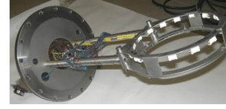
Figure 7: Set of 16 Mirnov coils mounted in a poloidal ring to work like sensors of local magnetic field.
