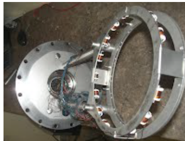
Figure 3.13: New set of local magnetic field sensors: 16 Mirnov coils circling the plasma column.
