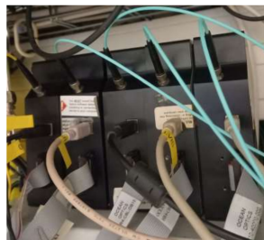
Spectrometers at GOLEM connected with the tokamak via optical fibers
