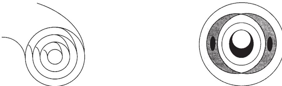
Figure 2.5: Ideally nested (a), and more realistic magnetic surfaces in tokamak (b).
