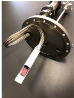
(b) PH32 detector attached to a radial manipulator, used during RE related GOLEM campaigns.
