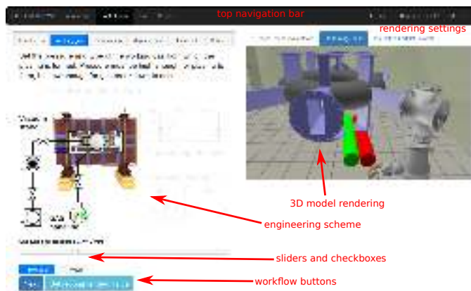
Fig. 2. Remote control interface of the GOLEM tokamak. The control room interface at the working gas setup step is shown.
