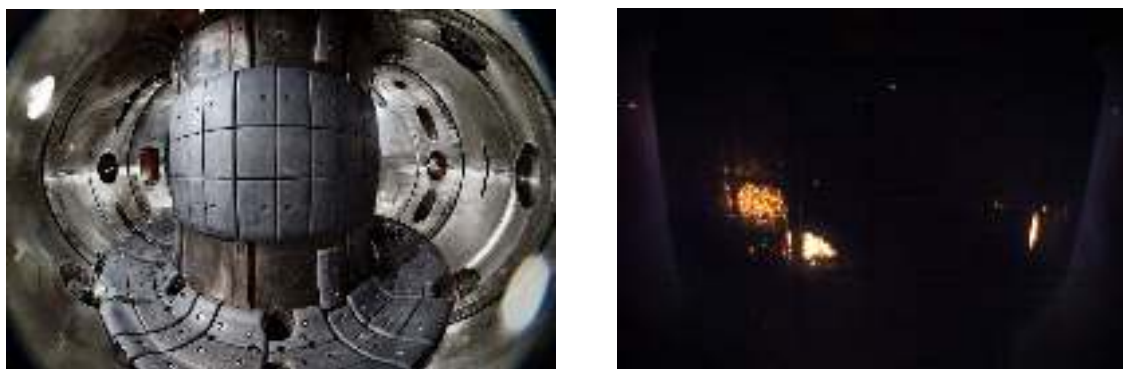
Figure 5. On the left, interior of the COMPASS tokamak vacuum chamber [18], on the right, shot 20056, snapshot taken at 991.3 ms from the fast camera Photron Mini UX100 operated at 6.25 kfps.
