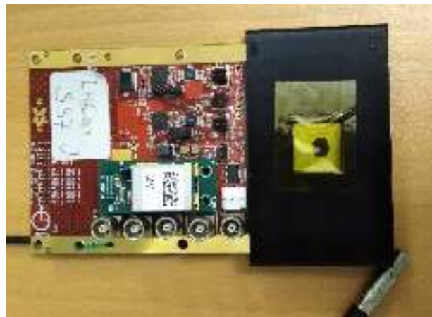
Figure 1: The Timepix3 chipboard. The hole in the Al layer on top of the sensor was cut out for laser experiments at Nikhef. The black plastic box around the sensor is used to shield the sensor from stray light and the yellow kapton tape keeps the sensor clean from dust.
