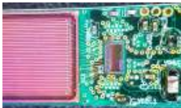
Figure 1. The silicon strip sensor connected to the PH32 readout chip by wire bonding.
