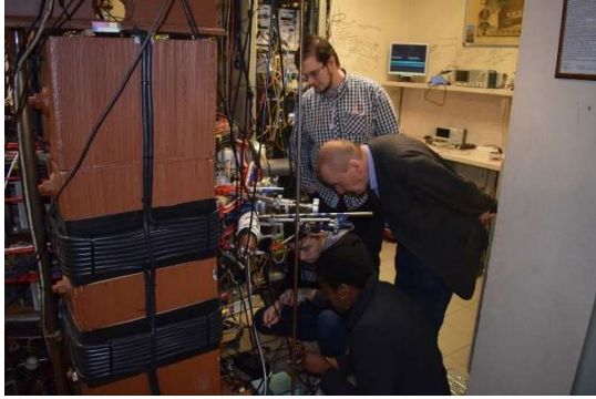
Naomi Mburu, Vladyslav Volkov and Georgii Sarancha adjusting the position of tunnel probe inside the GOLEM limiter with the help of RnDr. Jan Stöckel
