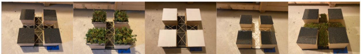
Photo 2: The 5 independent variable levels. From left to right: no mitigation strategy, green roofs, cool roofs, cool pavement, tree canopies (taken by student).
