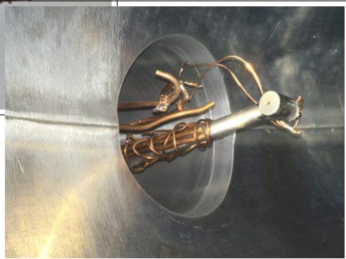
E-gun mounted inside the vacuum vessel
