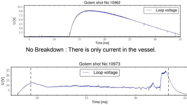
Breakdown : After some time, the loop voltage decreases, indicating that the resistivity decreases : the gas becomes a plasma, and carries a current.
