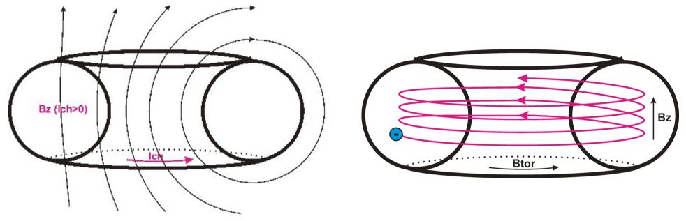
Free electrons will follow the magnetic field lines into the wall of the vessel, becoming then unable to start a cascade of ionization. This problem can be avoided by reducing the toroidal electric field, increasing the toroidal magnetic field, or increasing the pressure.
